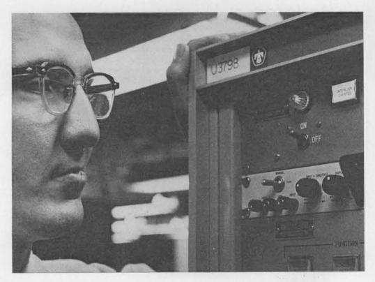
DEAN PEDERSON checks new safety system developed for production testers. The sign, "Interlock Cheated," lights up when the interlock safety system has been bypassed by someone working in the rear of the machine.
